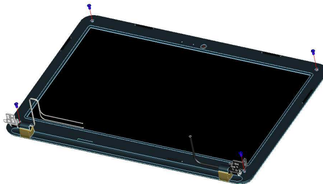
Figure 4-18-11 Secure the bezel with screws
