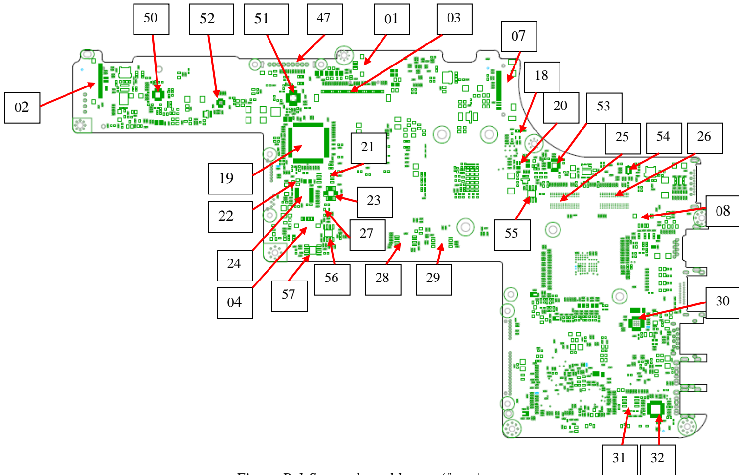
Figure B-1 System board layout (front)
