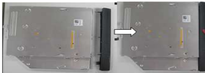
Figure 4-4-3 Assemble the ODD bezel
