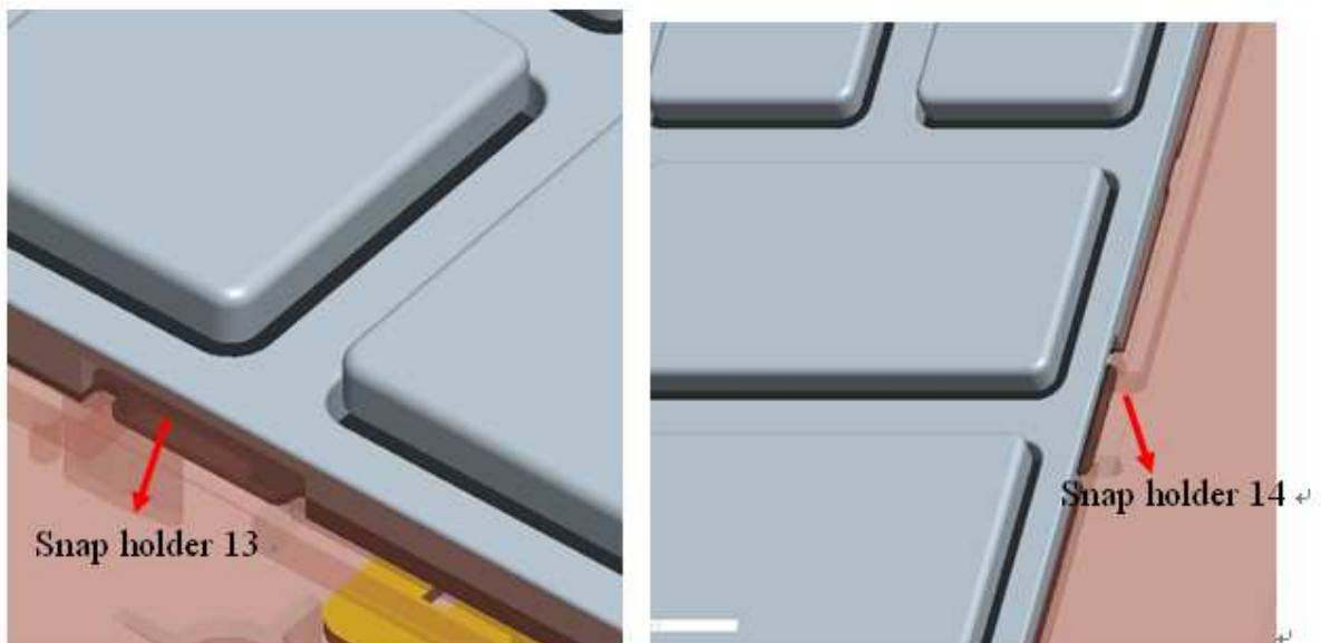
Figure4-7-4 Remove snap holder 13-14 and then remove the Keyboard
